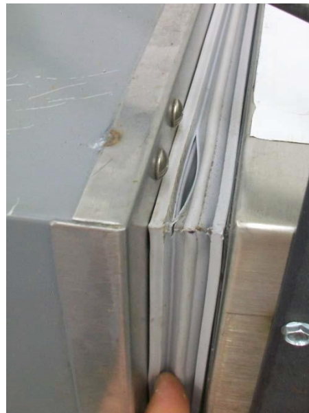
Gasket broken, need to be replaced
