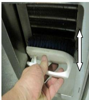
Use a soft bristled brush to clean greasy on the coil
